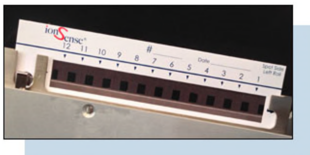
FIGURE 2: METAL MESH WITH TWELVE SAMPLE POSITIONS.
